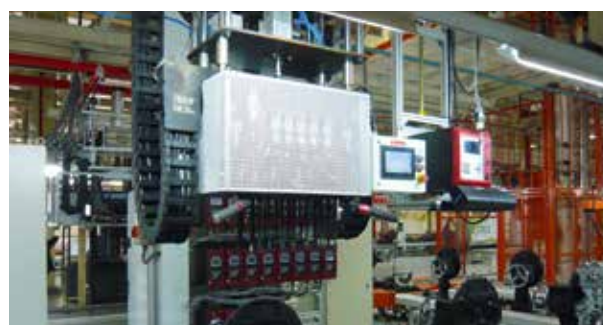
One power box supply with E Stop - Ethernet switches Multicombox - Circuit breakers
